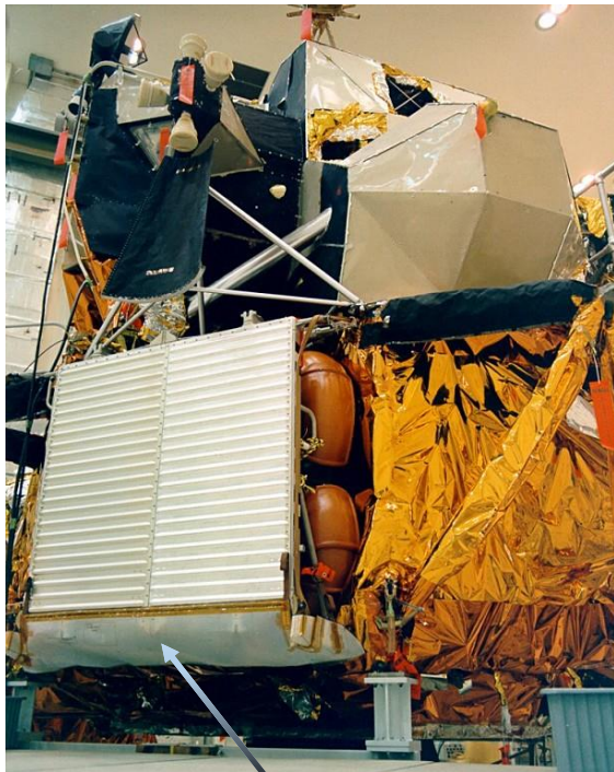
Kevlar Shield to Protect Rover from LM Lander Stirred Up Dust
